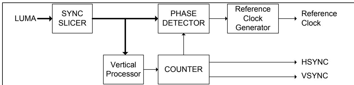
Figure 6-28 Synchronization Process
