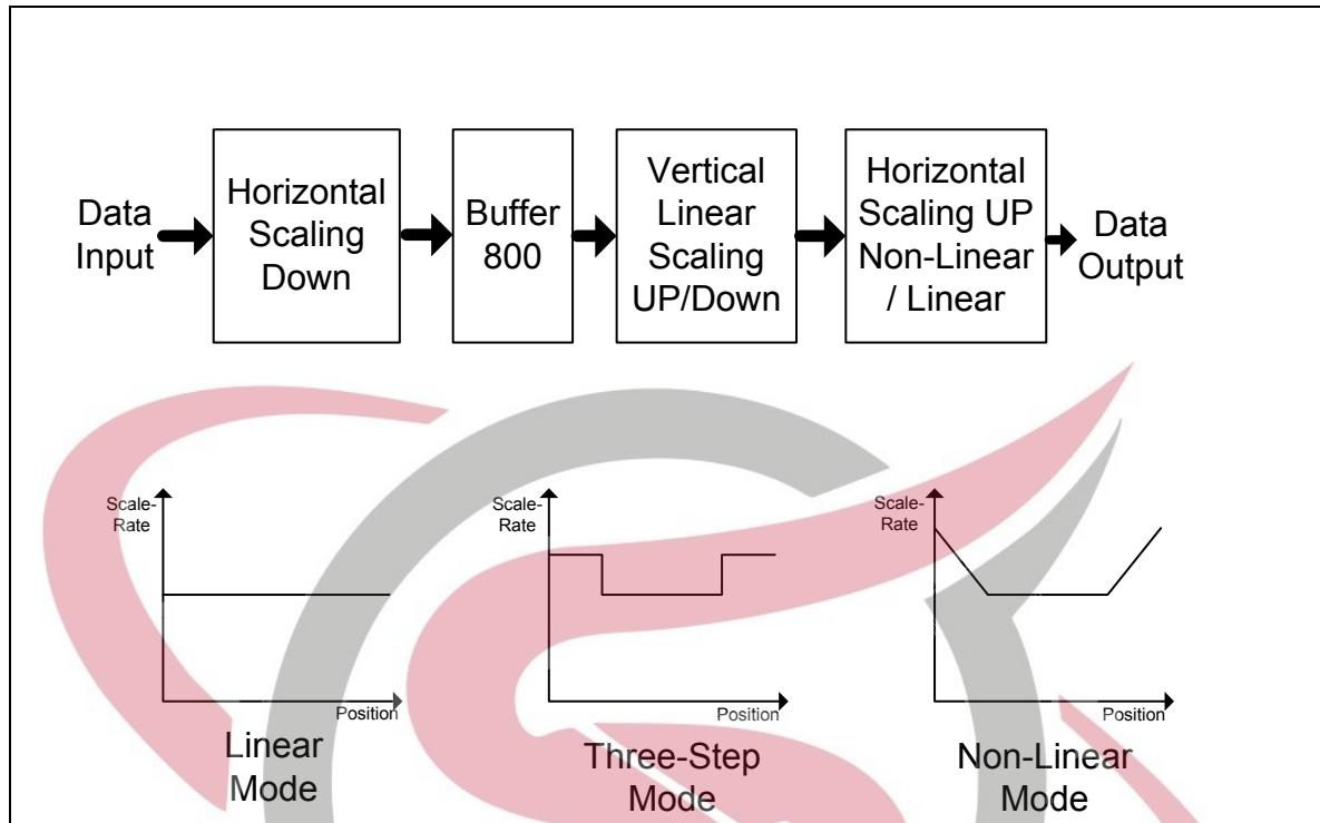
Figure 6-21 Scaling Function
